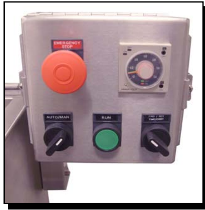
PLC BASED CONTROL PANEL
