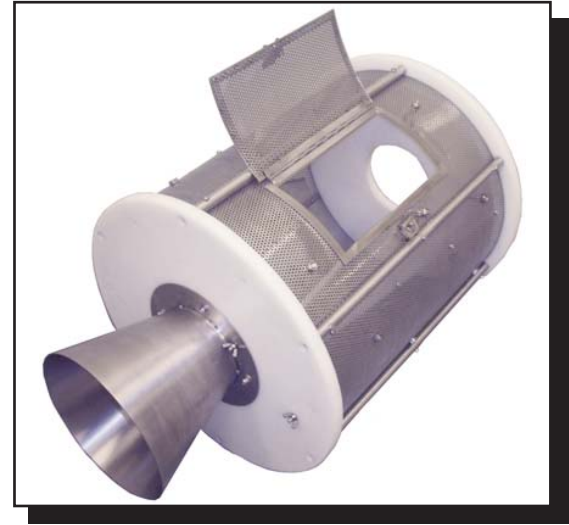
VIEW OF EXPOSED TUMBLE SYSTEM
