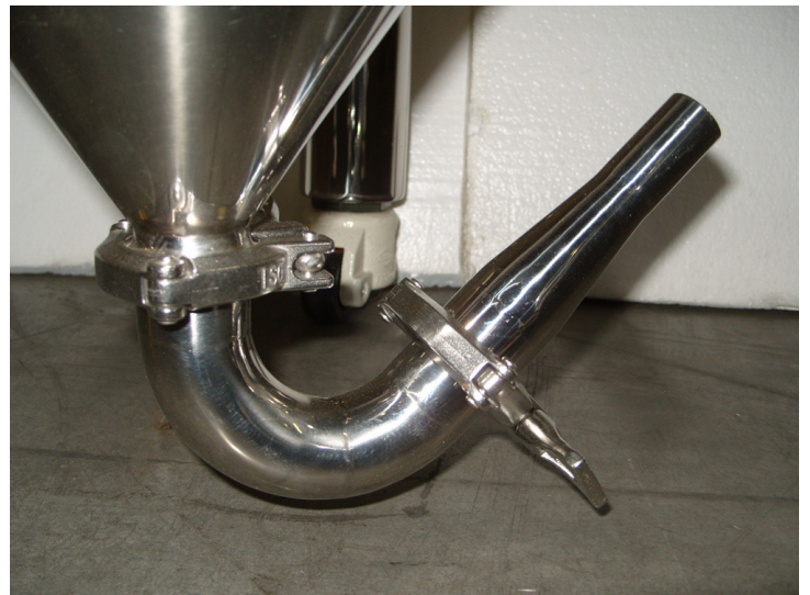
View of Bottom Discharge Leading to the Homogenizer
